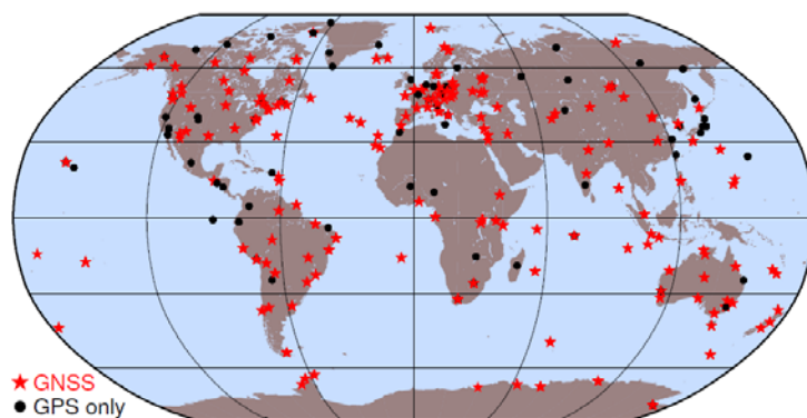
Geographical distribution of the IGS station network used in the current reprocessing activities (as of 2014).
