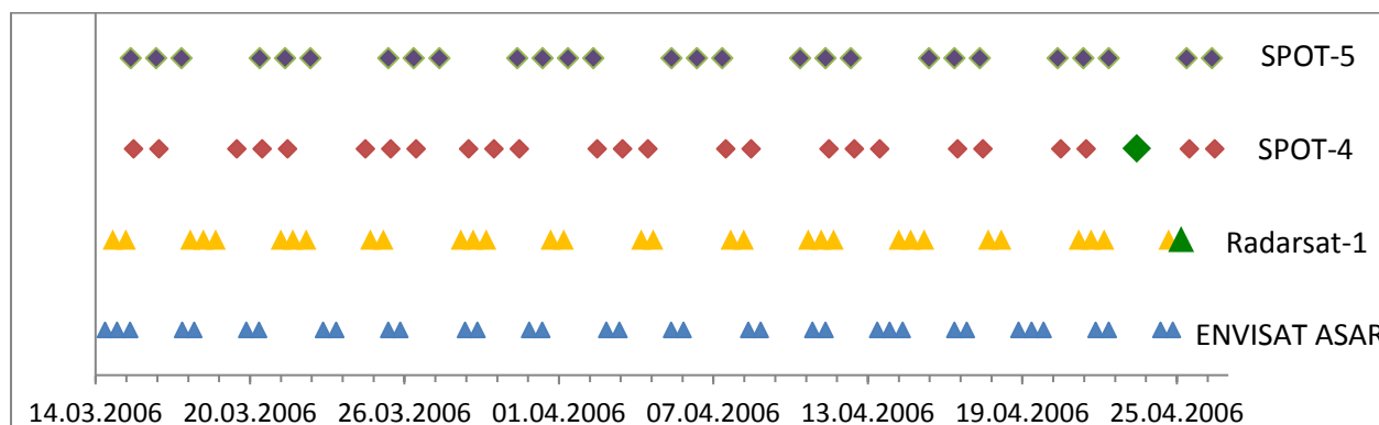
Figure 15: Possible overpasses and acquisitions of ENVISAT ASAR (wide swath mode with 150 m spatial resolution), Radarsat-1 (standard mode with 30 m spatial resolution), SPOT-4 (HRVIR sensor with 10 m spatial resolution) and SPOT-5 satellite (HRG sensor with 10 m spatial resolution) for the Danube delta region shown in Figure 5. Acquisitions that have been realized during Charter Call #121 are marked with dark green symbols.
