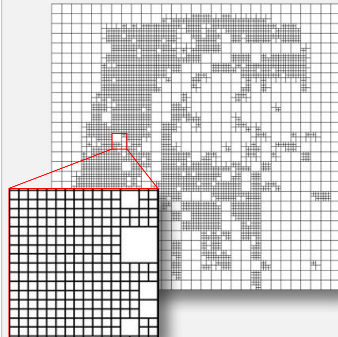
Sub-Tiles created by slope-dependent threshold
